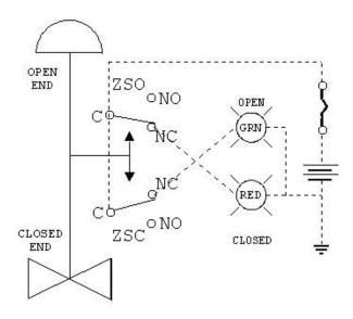
Figure 4 - Two limit Switches Failsafe
