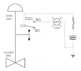
Figure 2 Single Switch, Direct Approach
